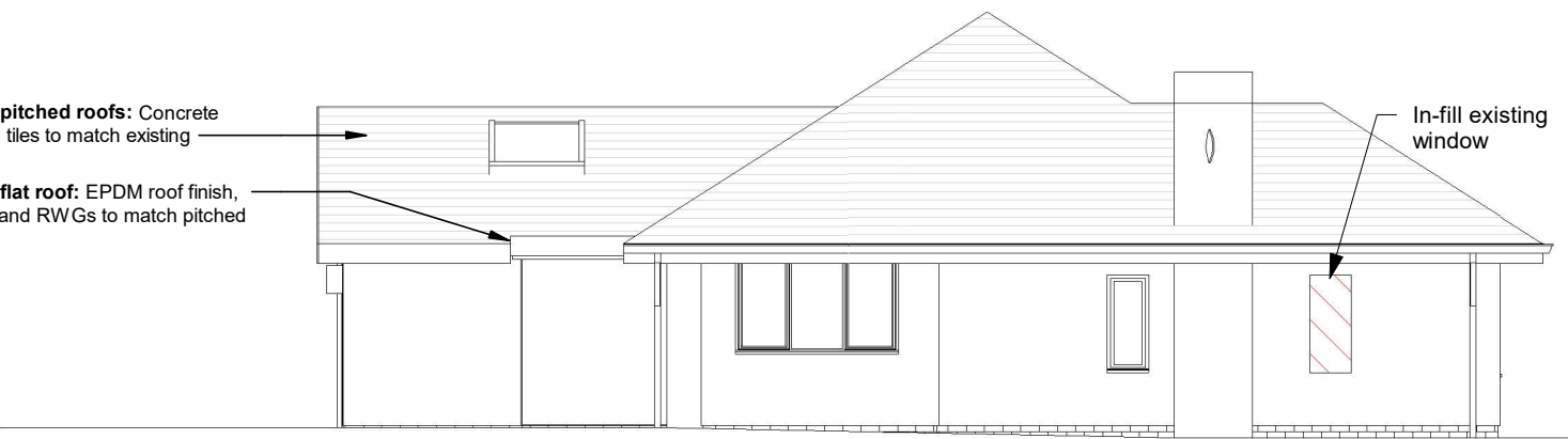
South West Elevation 1 : 100
