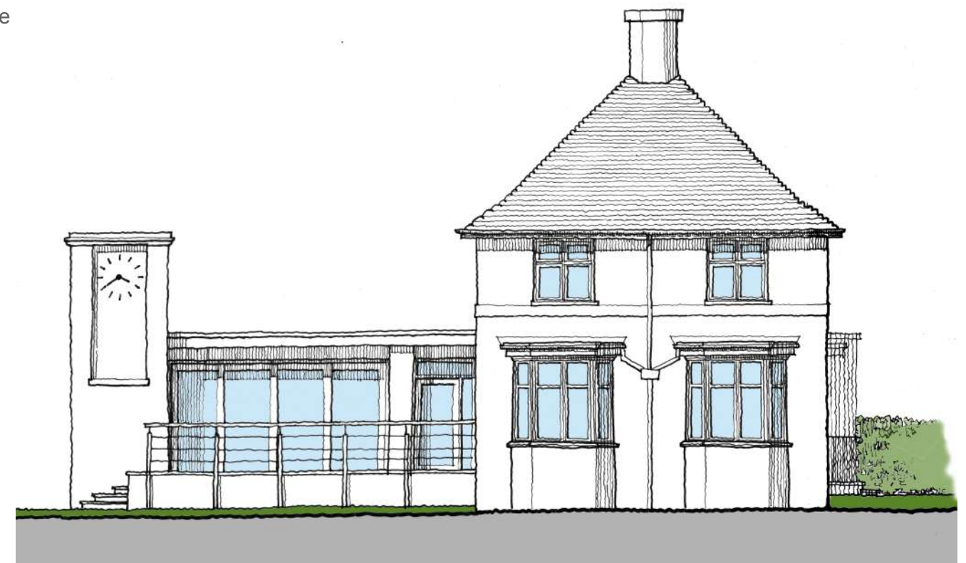
Above: An early concept sketch of the Lodge's proposed west elevation (not to scale). The new north extension (containing an open-plan seating area) is 'book-ended' by the proposed Clocktower and existing Lodge, left and right respectively. Portland stone detailing is proposed within the Clocktower and copings, additional space for external tables and chairs provided in front of the building (at both Cafe and Park levels).
