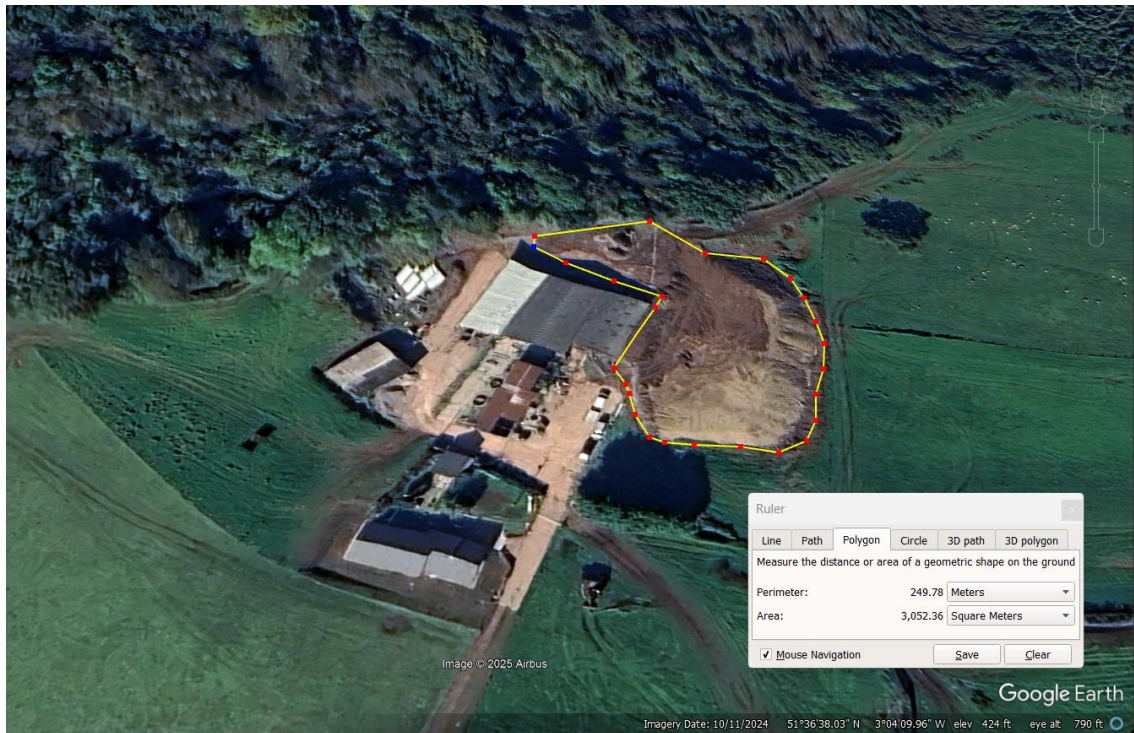
Figure 4, Aerial image showing earth works for ground levelling at Lower Wenallt Farm (Google Earth, June 2025)
