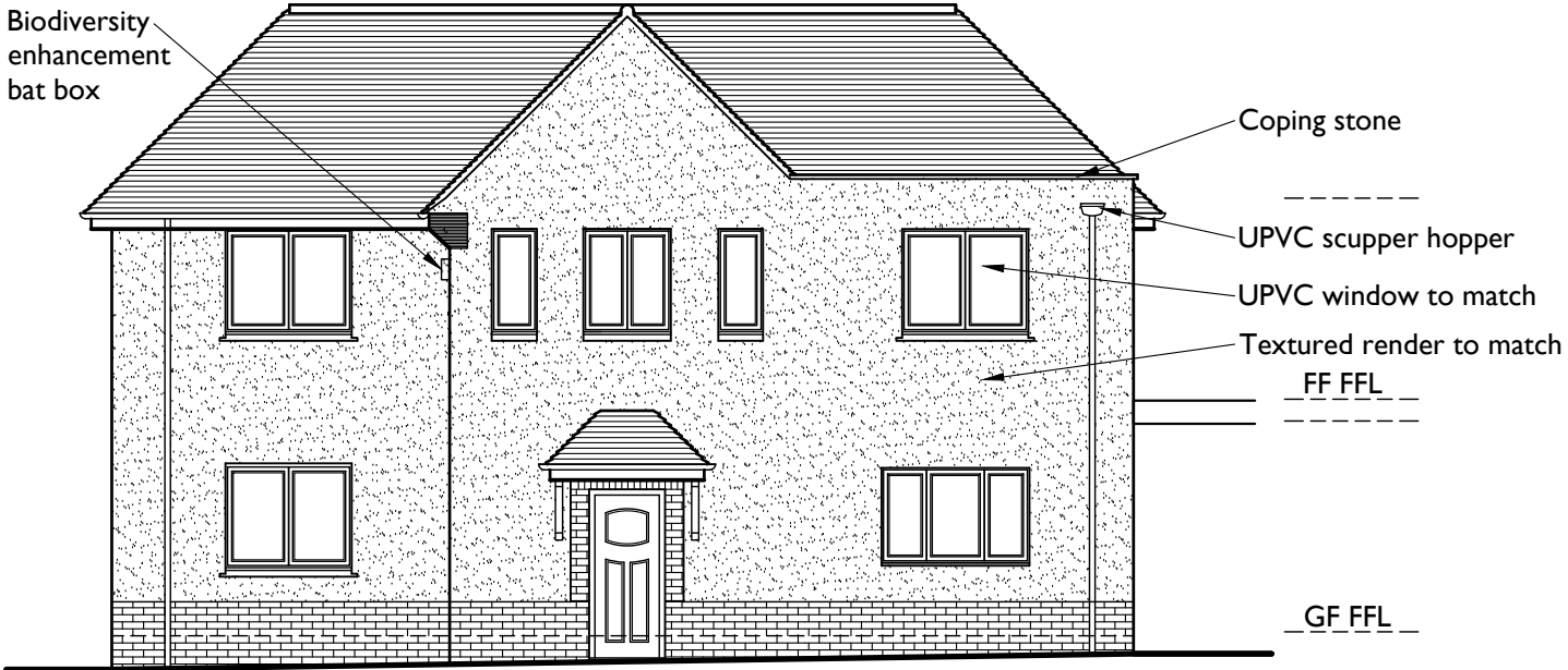
PROPOSED FRONT ELEVATION Scale 1:100
