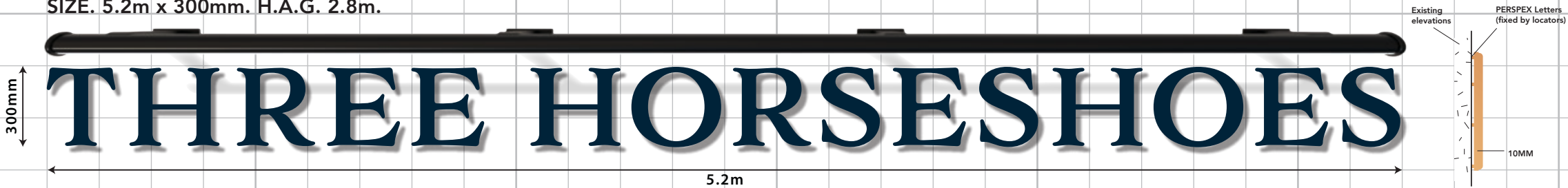
A ONE X NEW SET OF INDIVIDUAL LETTERS. NEW TROUGH LIGHT SIZE. 5.2m x 300mm. H.A.G. 2.8m.
