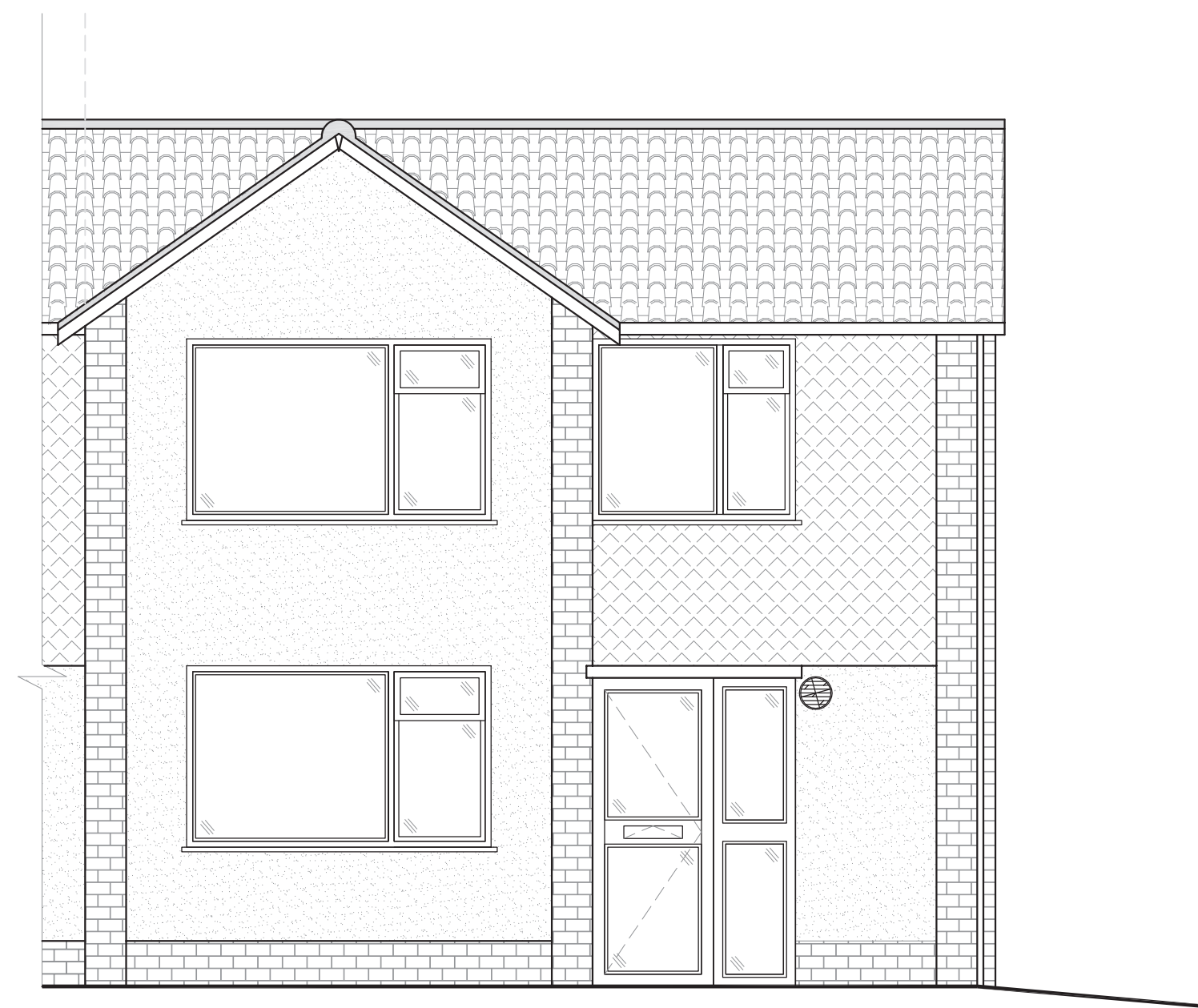
Existing Front Elevation
