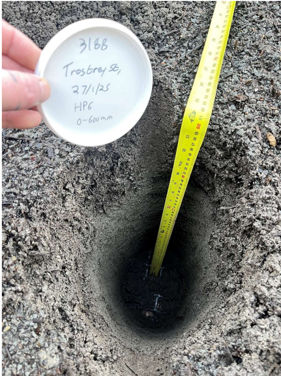
Hand pit excavated in the rear garden of Plot 6.
