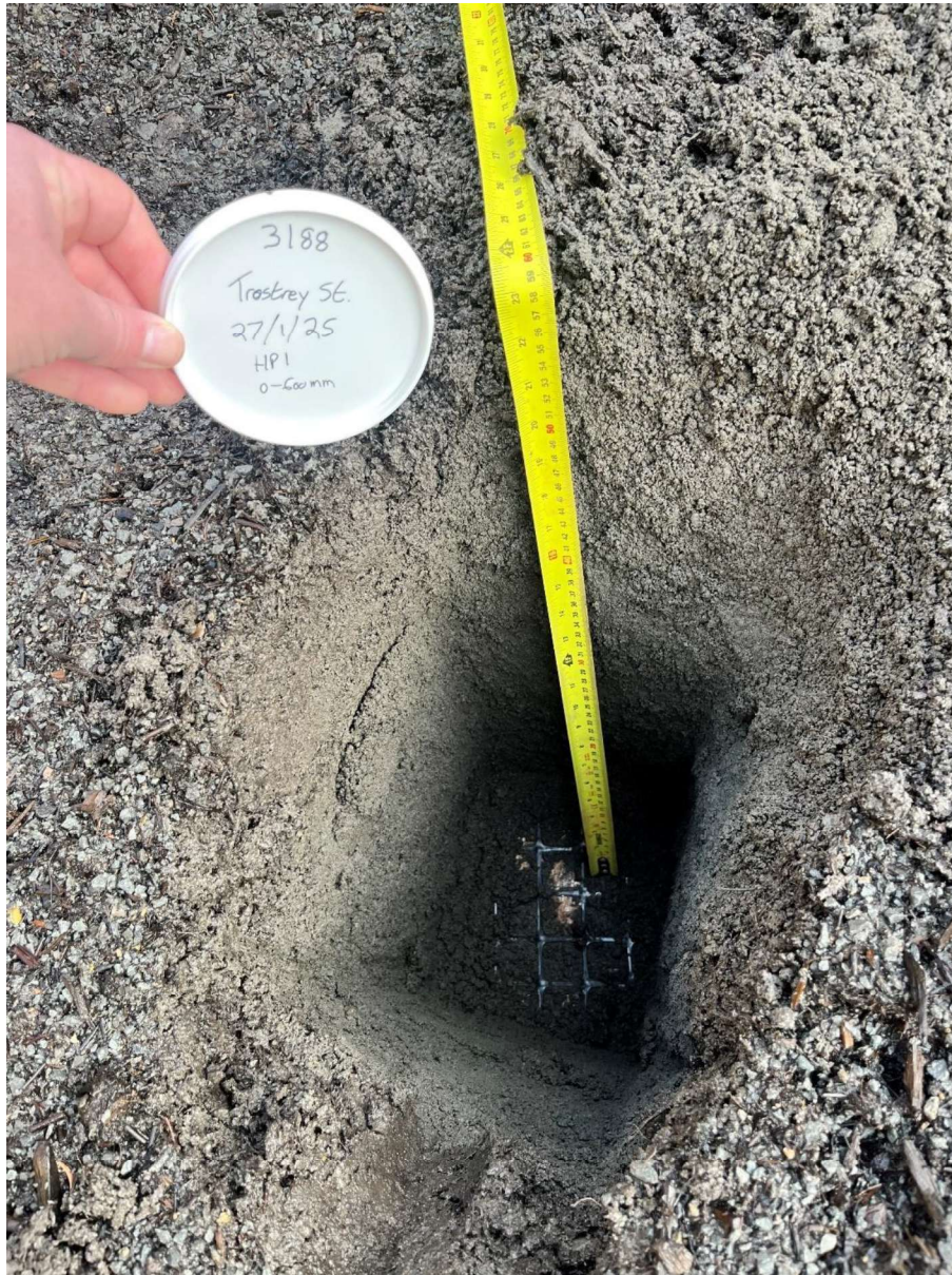
Hand pit excavated in the rear garden of Plot 1.
