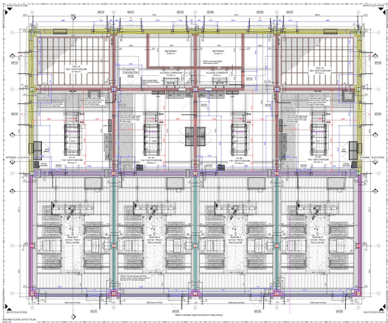
Figure 3: Proposed Transformer Locations in Substation
