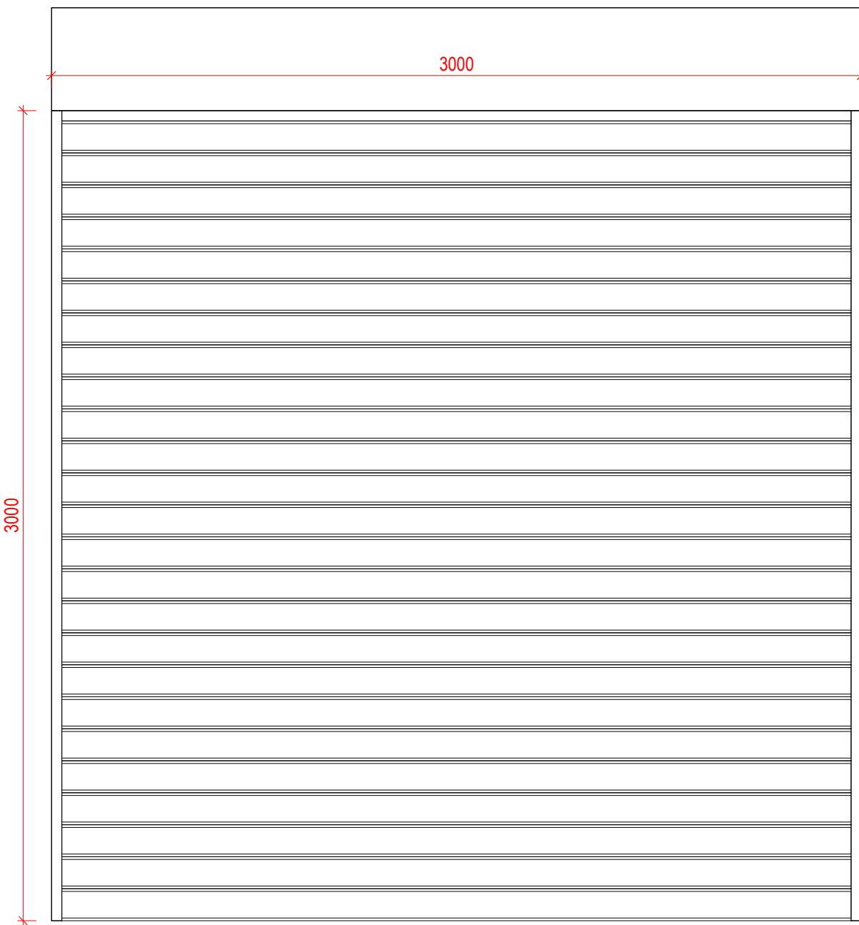
3No proposed new dock leveler doors Black RAL 9005
