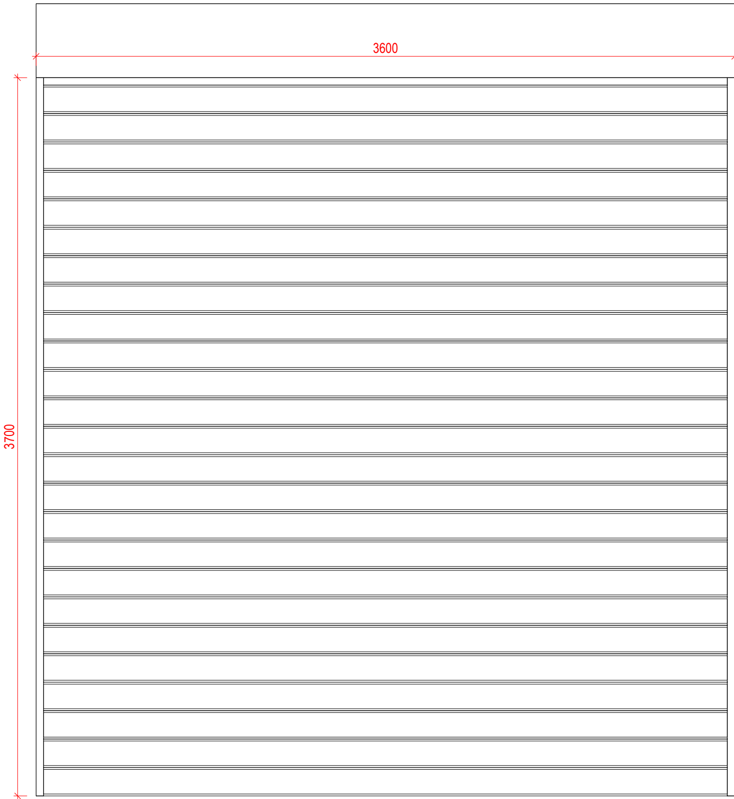
8No new proposed level access doors Black RAL 9005
