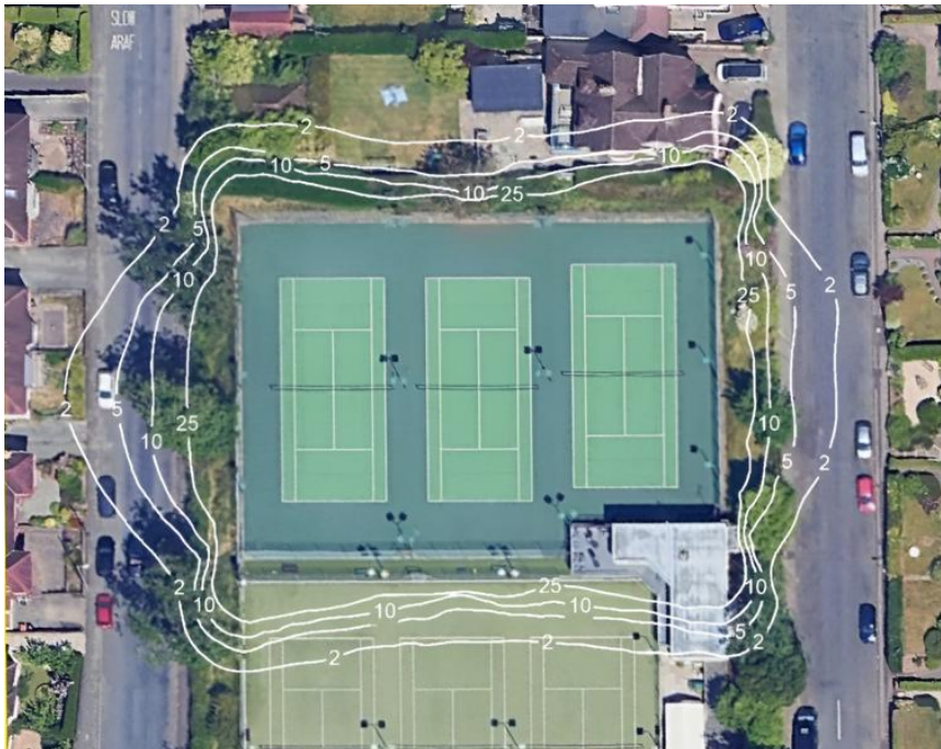
Figure 4: light spillage plan for LED lighting
