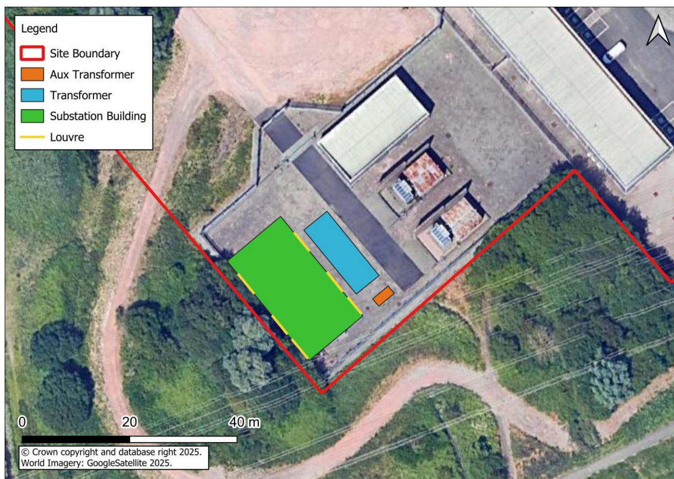
Figure 5.1: Assessed Plant Unit Locations
