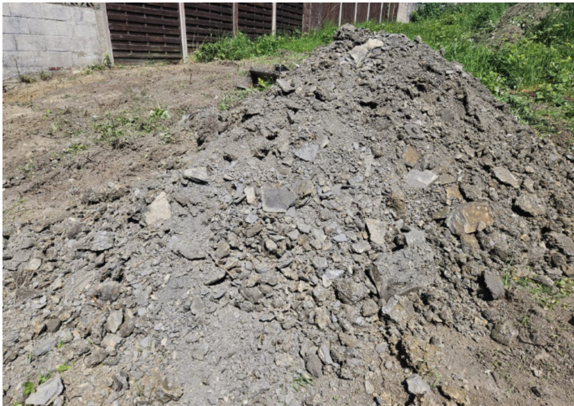
Dig material from pit. Compacted layers of sandy clay. Loose and friable once dug.
