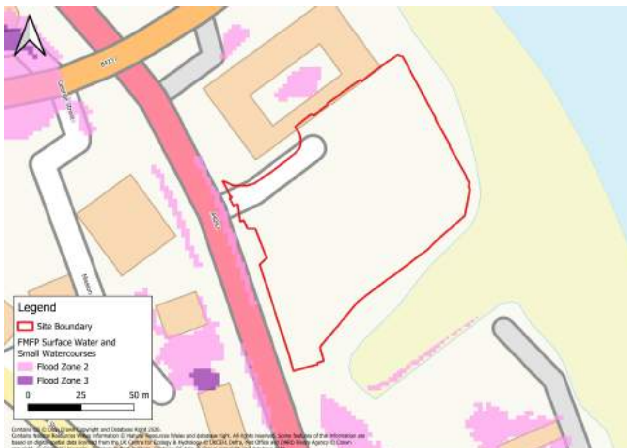
Figure 3-3 FMfP Flood Risk from Surface Water and Small Watercourses
