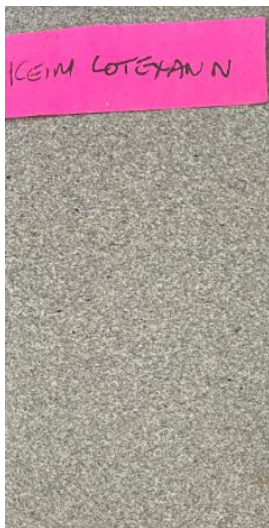
Plate 1: Treated stone with Keim Lotexan N
