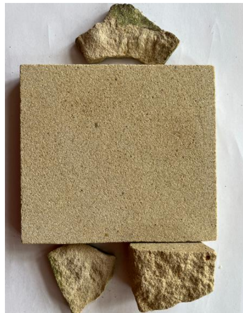
Plate 2: Witton Fell quarry, Buff sandstone matched to pieces of existing fallen stone at Shirehall.
