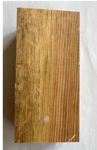
Plate 2: reclaimed pitch pine to scarf in
